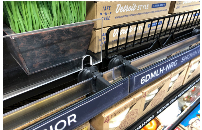
Cutouts in the plexi product stops provide clearance around the Ecoblade arms.
