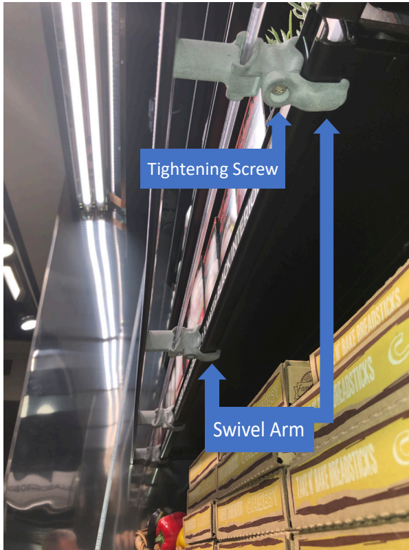
Bottom view of Ecoblade retrofitting to an existing shelf.
